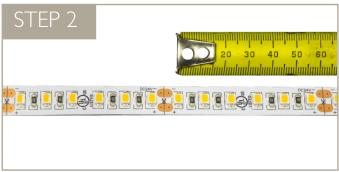
Remove the LED tape spool from its package and un-roll the LEDs.
