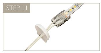
Pull the wires through the endcap(s) and remove red adhesive backing from the LED tape.
