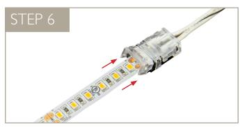
Make note of which wire is positive (+) and which wire is negative (-). Align the LED tape's positive and negative pads accordingly before inserting, then gently push the LED tape into the connector. Be sure to guide the tape over the pins inside the connector.
