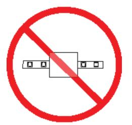
DO NOT COVER LED TAPE OR APPLY EXCESS PRESSURE TO LED TAPE
