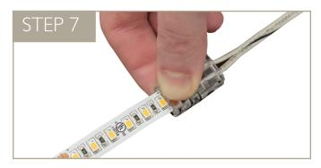
Tightly squeeze both ends of the gripper connector until the top covers click shut.
