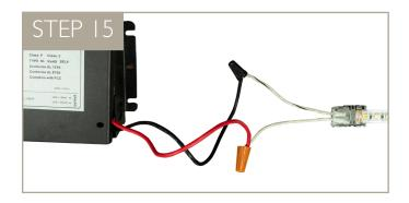
Connect the power supply to the LED tape wires. Make sure the connections are secure and correspond to the polarity of the LED tape.
