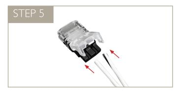
Carefully pry open the tops of the gripper connector, exposing the connection pins inside the connector on both ends. Insert wires into the larger end – do NOT strip wire.
