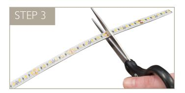
Cut the LED tape to the desired length. Make sure you cut along the marked line and that the cut is straight.
