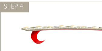
Peel back about a ¼ inch of the red backing and the adhesive tape, exposing the copper pads on the back of the LED tape.
