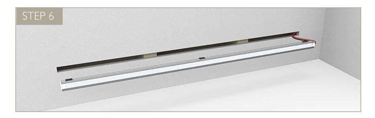
Route wires through opening. Install recessed mounting clips onto back of channel and insert channel assembly into opening.
