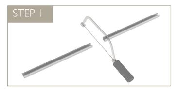
Measure the channel and cut to the desired length. Make sure to accommodate the profile of the endcap and the desired length for your LED tape before cutting.
