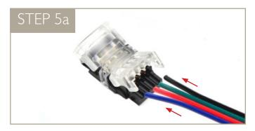
Carefully pry open the tops of the gripper connector, exposing the connection pins inside the connector on both ends. Insert wires into the larger end – do NOT strip wire.
