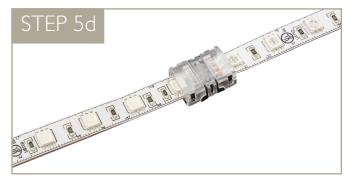
Use the LED-to-LED gripper connector if you are interconnecting LED tape sections. Be sure to align section's positive (+), Red negative (R-), Green negative (G-), Blue negative (B-) and White negative (W-) connections.
