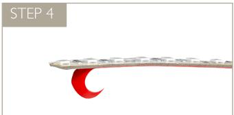
Cut the Linear LED to the desired length. Make sure you cut along the marked line and that the cut is straight.
