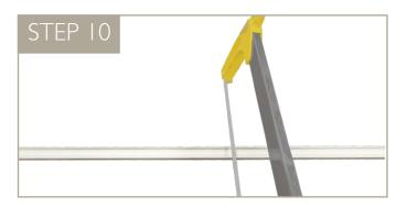
Measure the channel to verify that it is the appropriate length. Cut the channel if needed.
