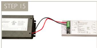
Open both wiring compartments on each end of the 4-channel receiver.
