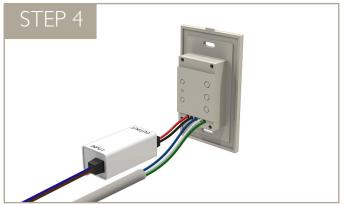
Connect data wires to controller data input terminals. Use green wire for GND, blue wire for D(-), white wire for D(+).
