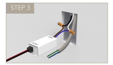
Connect power supply input wiring to line voltage and place inside wall box.
