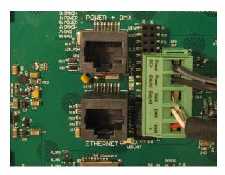
**NOTE:** Do not apply power to the DMX screw-terminal input. Doing so will damage the controller and void the warranty.
