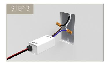
Connect power supply input wiring to line voltage and place inside wall box.
