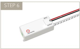
Once your controller is powered up, momentarily press and release the learning key on the RF receiver.
