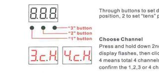
Through buttons to set desired DMX512 address, click button 1 to set "hundreds" position, 2 to set "tens" position, 3 to set "unit" position.
