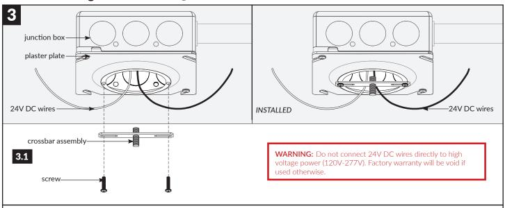
3.1 Align the crossbar assembly to the junction box plaster plate holes and secure using two #8-32 screws. Be careful not to pinch power wires between the crossbar assembly.
