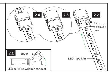
3.1 Carefully open the wire cover on the LED to Wire Gripper connect.
