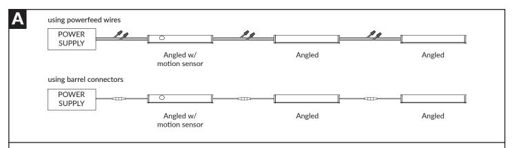
A. When connecting multiple units to each other, make sure to connect the unit with the motion sensor first. Followed by connecting the other units afterwards, that way the unit with the motion sensor turns on. Then the others will turn on automatically.
